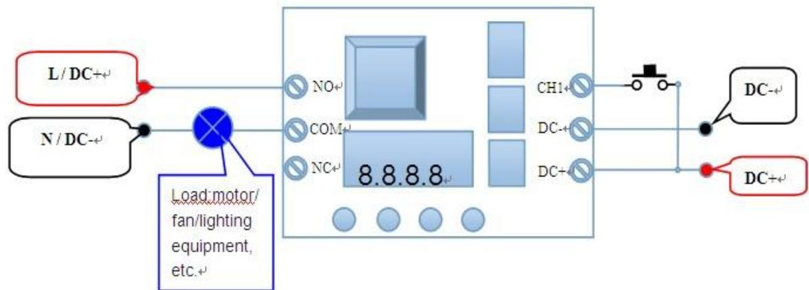
**Gentle remind:** If user load and FRM01 module use a seam DC power supply, it is possible because of the power supply capacity is insufficient or wiring connections unfit, the module appears unstable phenomenon occasionally, please use the following (even if no found the problem, it should follow the recommendations):
